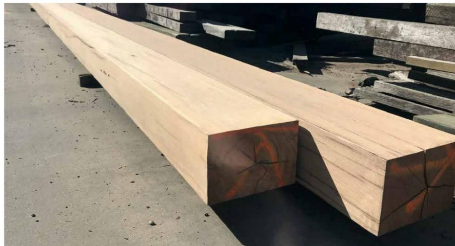
Above: Demolished Australian bridges, warehouses and more provide a great source of visually appealing structural hardwood timbers, such as these 11.8m Ironbark beams.
